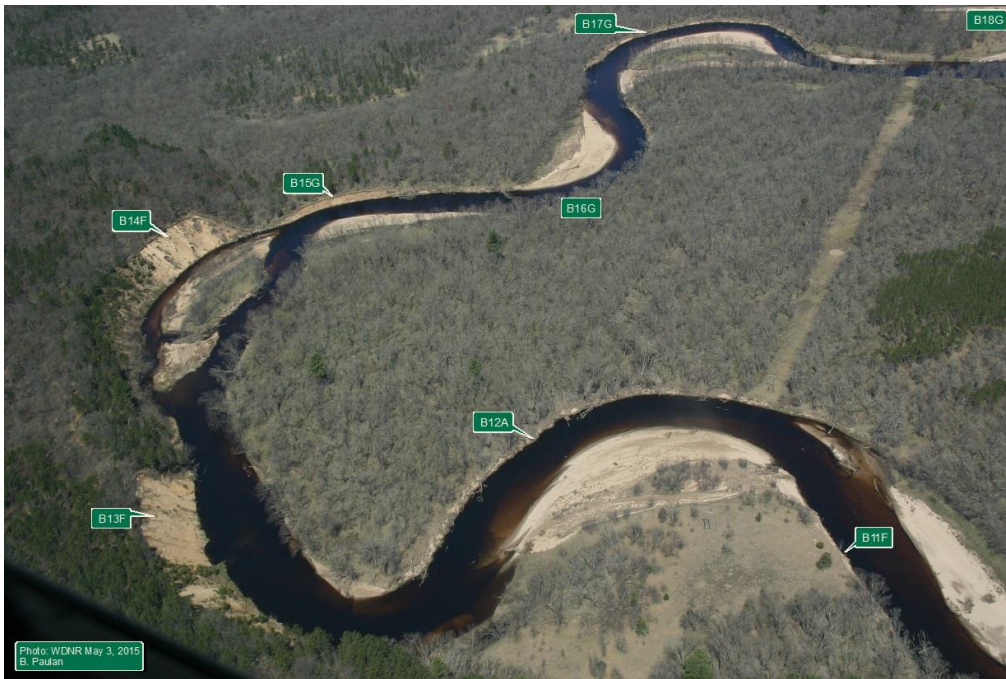
Figure 3: Low Altitude Aerial Photograph of Stretch of Lower Eau Claire River with Identified Erosion Sites from Table III
